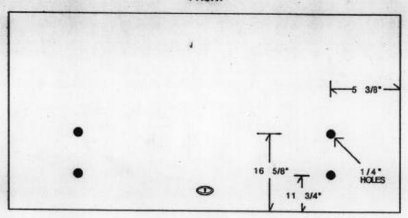
Measurements are taken using the edge of the deck lid above the taillights as the starting point. Follow the contour of the decklid with a measuring tape to the correct dimension. Drill a 1/4" hole for the studs.
